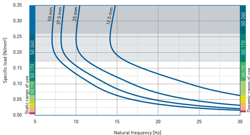
Natural frequency of a single-degree-of-freedom system consisting of a fixed mass and an elastic bearing consisting of PURASYS **vibrafoam** SD 170 on a stiff subgrade.
