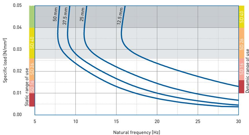
Natural frequency of a single-degree-of-freedom system consisting of a fixed mass and an elastic bearing consisting of PURASYS **vibrafoam** SD 26 on a stiff subgrade.
