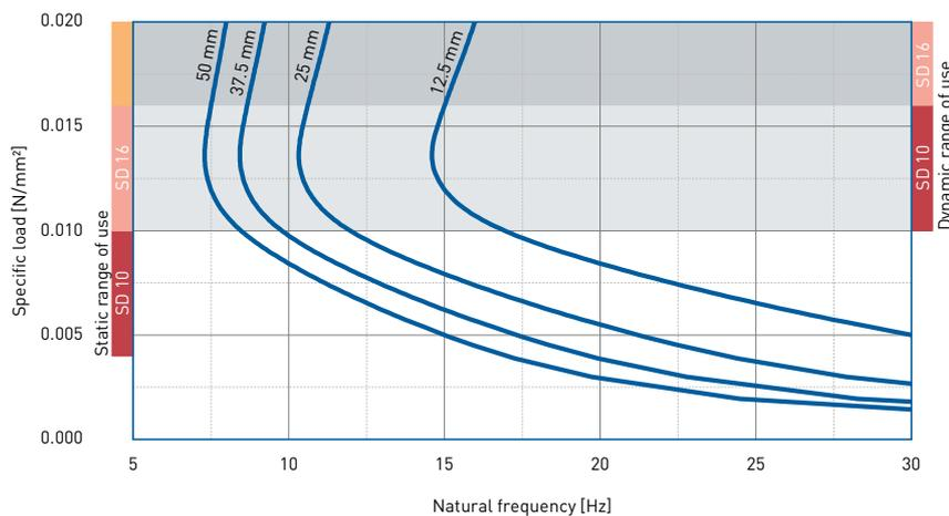
Natural frequency of a single-degree-of-freedom system consisting of a fixed mass and an elastic bearing consisting of PURASYS **vibrafoam** SD 10 on a stiff subgrade.
